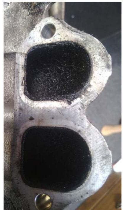
Cleaning out this assembly is a messy old affair so be warned! Use a screwdriver to scrape out as much solid debris as possible and then the wire brush to get back to metal. Try and get into as many areas as possible but be careful to avoid doing damage to the mating surfaces.
