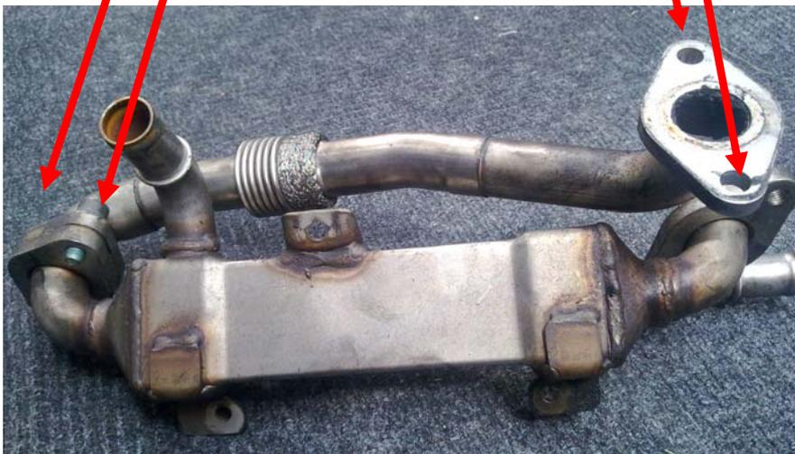
With this pipe removed you now have access to the 3<sup>rd</sup> retaining bolt of the EGR Valve which is next to be removed. Disconnect the two vac pipes going into the valve (red) and the bolts (green) – again they are tricky to access. Lift out the EGR valve assembly.
