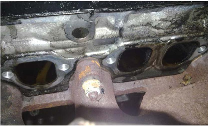
With the manifold removed it's now time for the cleaning and de-gunking of the assembly. It's easy to forget this stage later on so start by using a clean rag to wipe around the back of the cylinder head against where the gasket will seat. Care should be taken that nothing falls into those inlet ports including debris and solid particles from the surrounding area but a clean surface is essential for a good seal when the unit is refitted.
