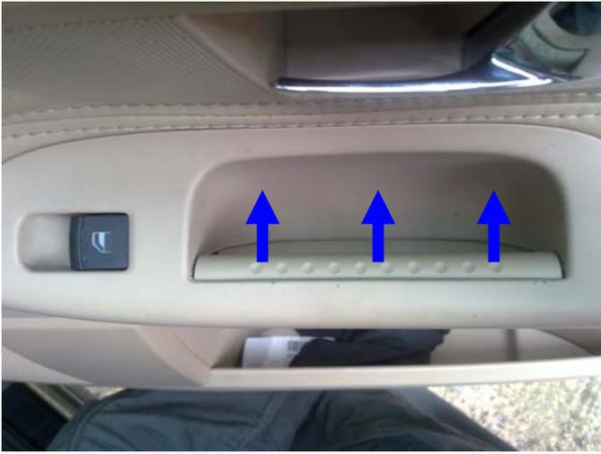
So to removal, the first thing to do is prise out the inner door handle support. This allows the door handle to be removed and access to the retaining bolts.
