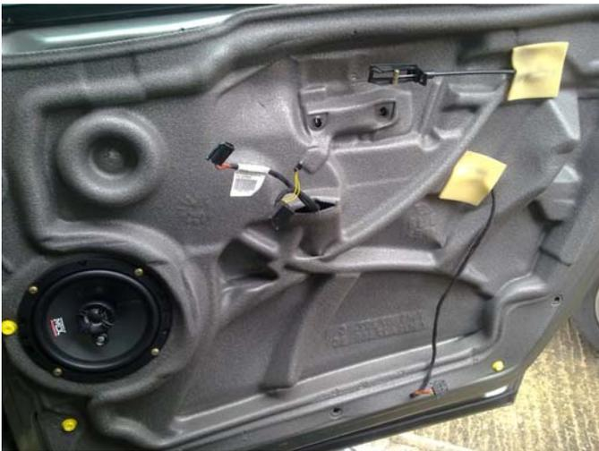
Remove the speaker next, 4 screws will allow the speaker to pull forward and the connector be disconnected. Remove left over clips at this stage!
