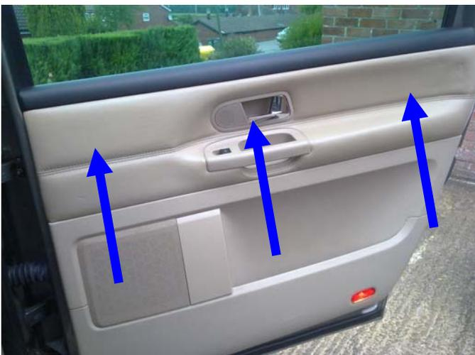
With the bolts removed the door card now pulls out slightly at the bottom and then lifts up to clear the hook bar at the top. Note this can be the trickiest part as the clips hold the card tight to the door frame. Be careful not to pull the door card outward too much as the clips are held onto the card by a plastic piece which is simply glued to the card.
