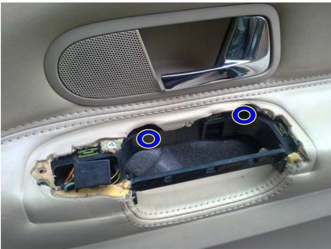
Finally disconnect the wiring to the window switch and remove the handle assembly. You can now access the two 10mm bolts that are the primary fixings for the door card and remove them.
