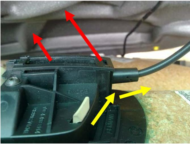
With the card lifted off the hook bar, you need to release the door opener and disconnect the wiring for the tweeter and open light (if fitted)
