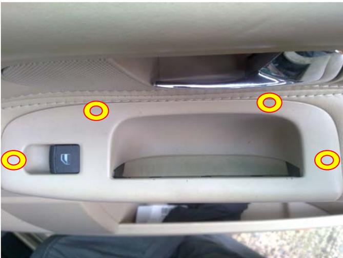
Once it's removed the handle surround can be lifted up – note its only held by 4 spring clips as shown in picture 2.
